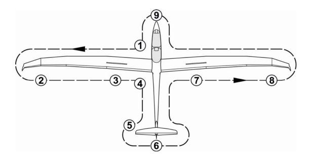
When walking around the aircraft, check all surfaces for paint cracks, dents and unevenness. In case of doubt, ask an expert for advice.
