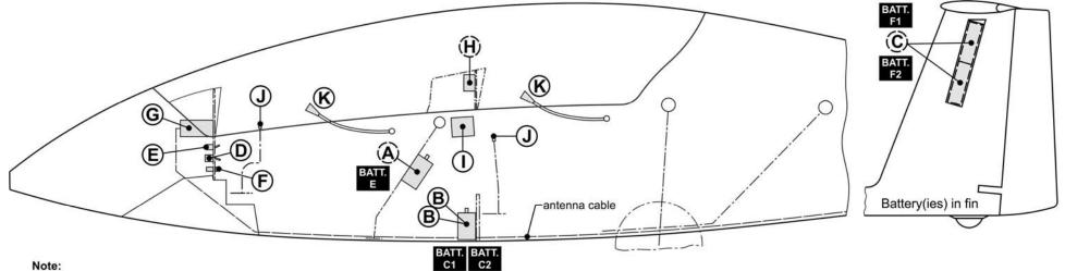
VHF-Transceiver and other additional equipment to be wired in compliance with the manufacturer's instructions and be fused individually.
