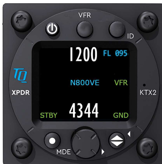
GND-switch installed, on GND
