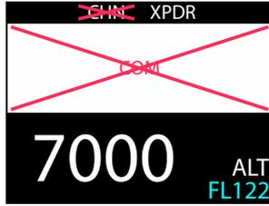
Figure 8.2.: No data/communication with connected COM system.
