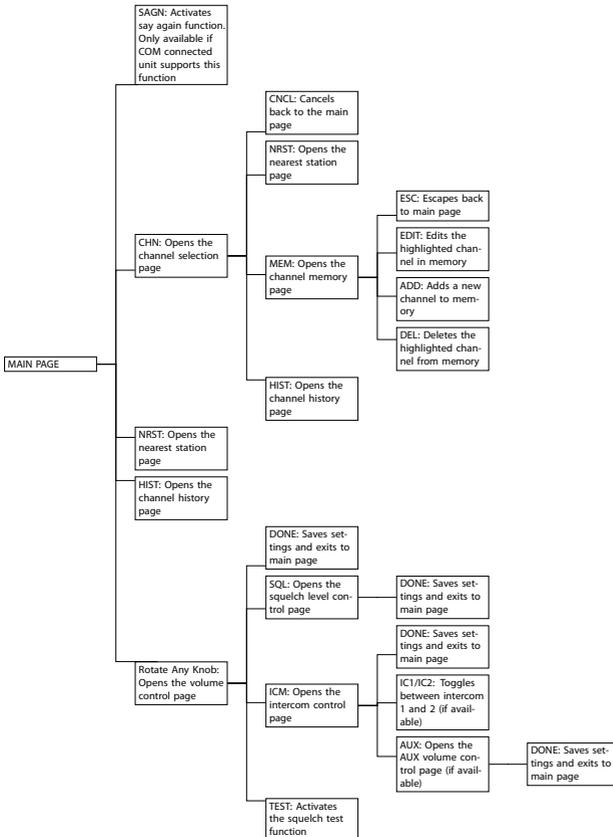
Please note that depending on the setup of the *KNOB USE* parameter, the **CHN softkey** on the main page may be replaced by a **VOL softkey** (volume control) and rotation of **inner knob** or **outer knob** will open the channel selection page.
