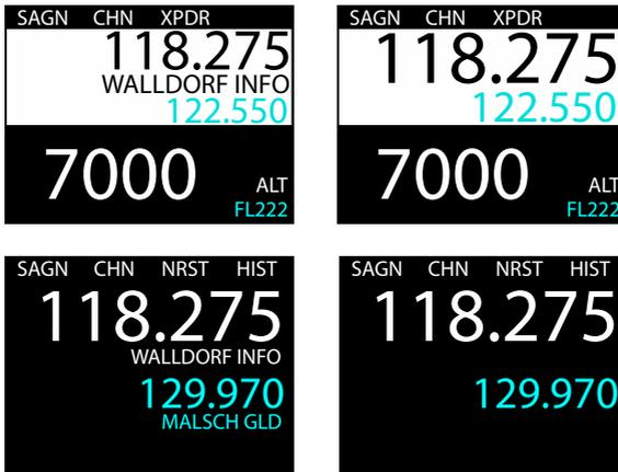
Figure 6.2.: COM main page with *STATION NAMES* parameter set to *ON* on the left and to *OFF* on the right. Please note that in COM only configuration, station names for both standby and active channel are shown. In all other configurations, only the active channel station name is shown.
