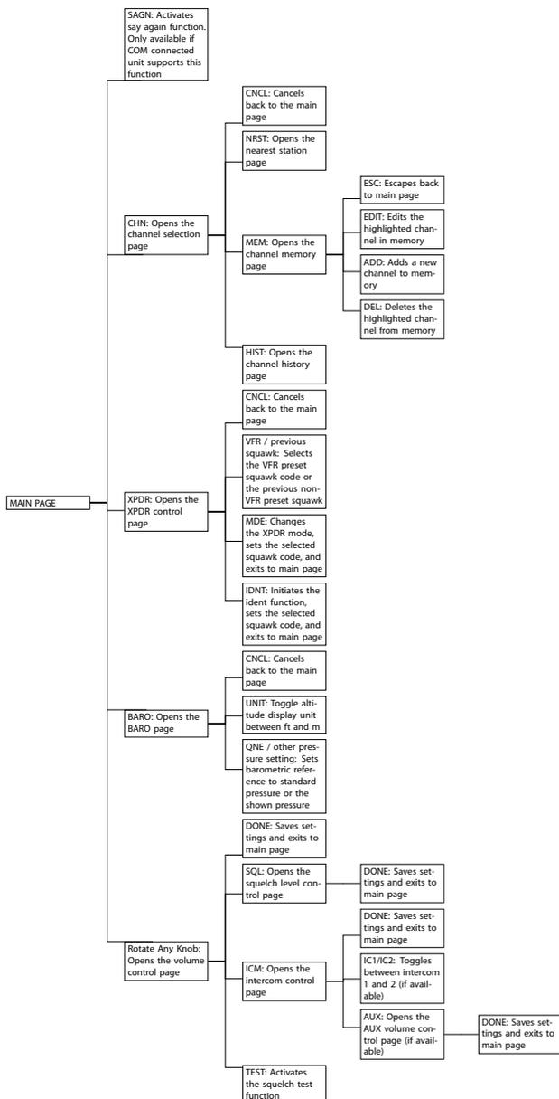
Please note that depending on the setup of the *KNOB USE* parameter, the **CHN softkey** on the main page may be replaced by a **VOL softkey** (volume control) and rotation of **inner knob** or **outer knob** will open the channel selection page.
