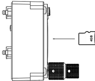
Figure 7.2.: microSD card in correct orientation
