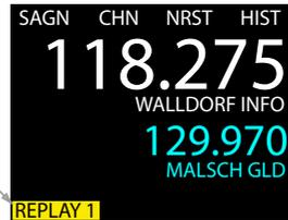
Figure 2.17.: **SAGN softkey** has been pushed, replay function is active
