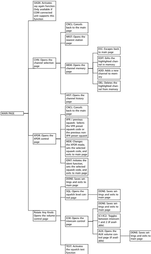
Please note that depending on the setup of the *KNOB USE* parameter, the **CHN softkey** on the main page may be replaced by a **VOL softkey** (volume control) and rotation of **inner knob** or **outer knob** will open the channel selection page.
