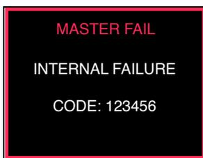
Figure 8.1.: Major internal failure annunciation
