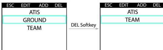
Figure 2.13.: Channel deletion process in channel memory list
