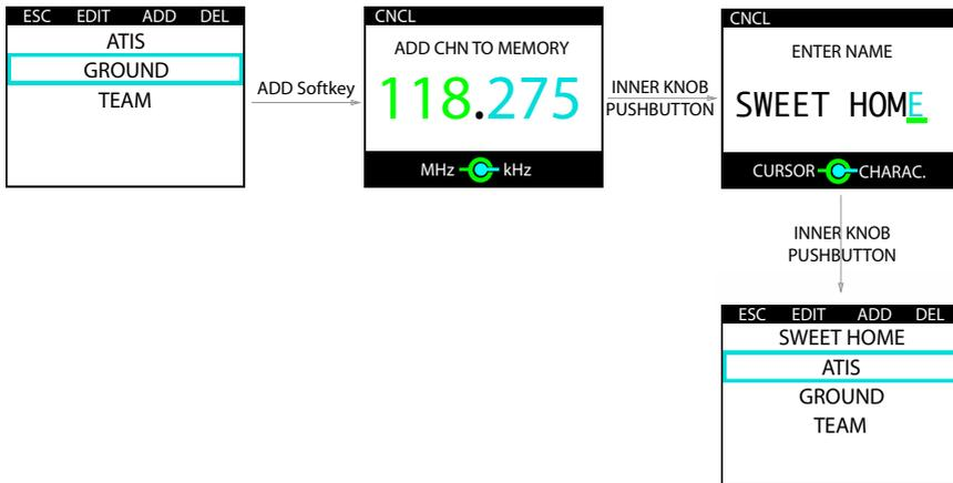
Figure 2.11.: Channel storing process in channel memory list
