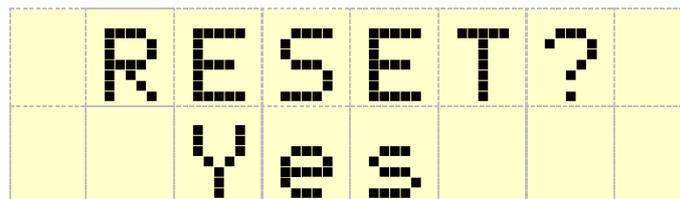
The reset process is activated by pressing the SET button. The reset is confirmed with "DONE" and the transceiver automatically restarted
