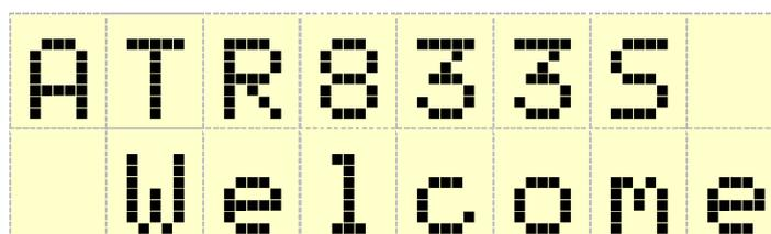
The start screen indicates the device type. After that screen the device changes into normal operation (direct input mode).
