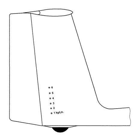
Water ballast is <u>dumped</u> from the fin tank through an opening on the <u>lower</u> side of the fuselage tail boom, adjacent to the rudder.
