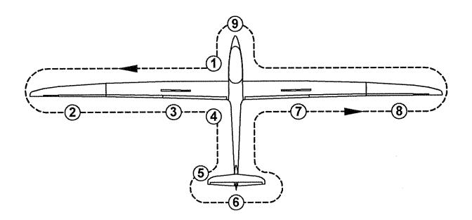
When walking around the sailplane, check all surfaces for paint cracks, dents and unevenness.
