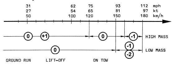
Only small control surface deflections are necessary to keep station behind the tug.
