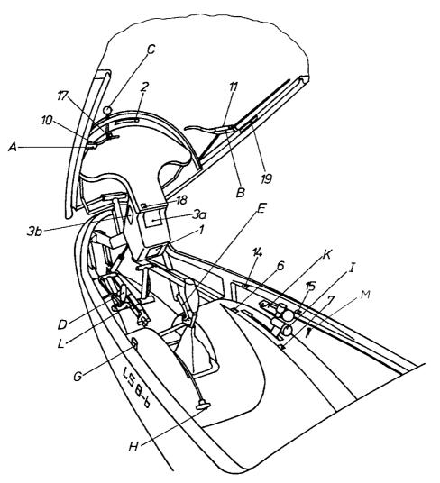
Numbers refer to placards, see also Flight Manual, section 2.12.1 and Maintenance Manual section 7
