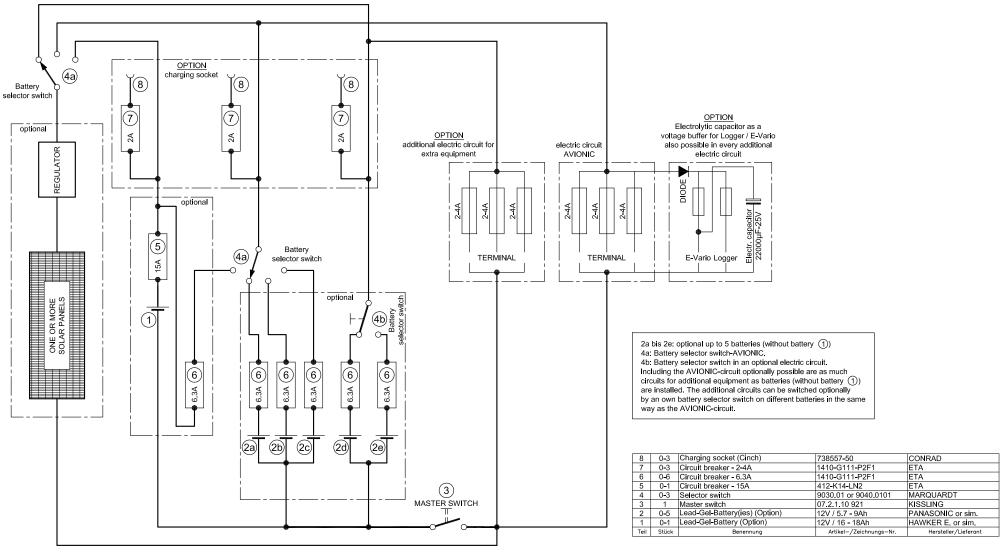
Solar panels to be wired at the main power supply only by regulator with V<sub>max</sub> = 13.8V **WIRING DIAGRAM**
