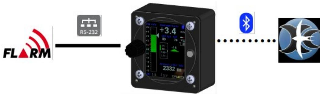
The RS232 interface is used either to connect a device without wireless (Bluetooth or WiFi) support (OpenVario, older Kobo), or to connect a FLARM as shown above.
