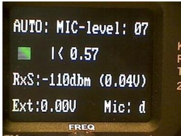
The MIC submenu is terminated by pressing the AUD button.
