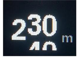
This item allows you to choose to what extent the altimeter display is quantized to an interval of 2-20 meters (or 6-60 ft), as shown in the graph to the right with 10 meters. The two digits then move up (rise) or down (fall) like on a counter wheel, which significantly improves readability when the flight altitude is in motion compared to the simple digital display.
