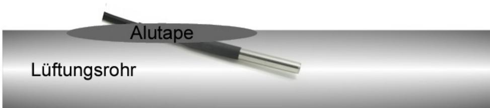
This can also be done in the ventilation pipe if available. In this case, a small slit is cut with a cutter knife, the temperature sensor is pushed in and sealed with aluminum adhesive tape or silicone, for example.
