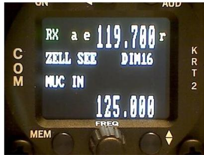
The display consumption at 12V is between 10mA und 70mA. In addition the battery voltage in Volts is indicated.
