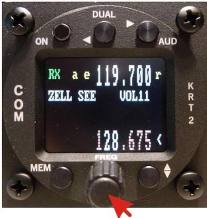
The Standby-Frequency is set with the turning knob in 3 different ranges. The selected range is highlighted and can be changed with the **FREQ** button. Frequency ranges are:
