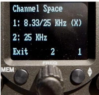
The desired channel spacing then can be selected and the (X) then indicates the actual channel spacing.
