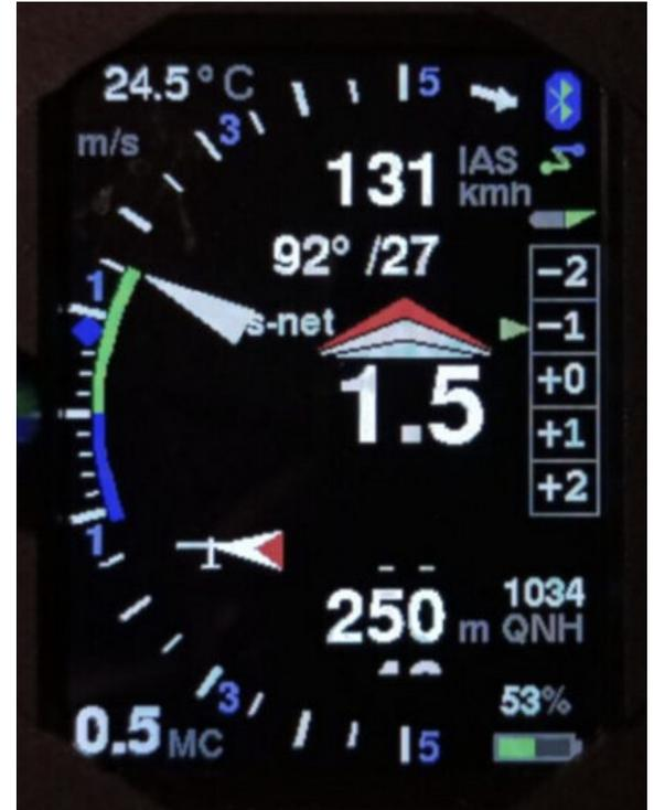
The altimeter can be displayed in full resolution or quantized to 10 meters as shown here in the form of a sliding scale.
