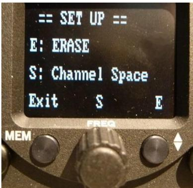
To exit the SET-UP menu, use the MEM button. The unit remains powered and the normal operating mode is resumed.
