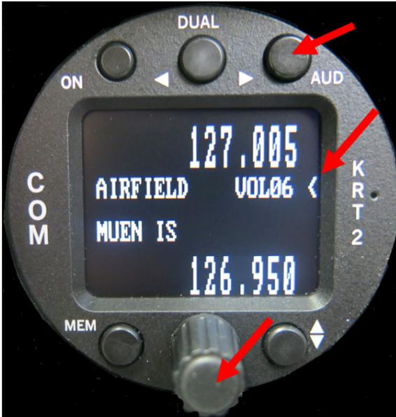
Any action in the Audio Menu requires the pointer (<) to be next to the Audio menu window (see picture). When the pointer is next to the Standby frequency window, the pointer can be repositioned by pressing the AUD button once.
